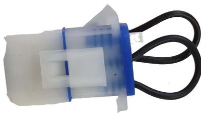
For this reason it is always necessary to insert the closing connector (male connector with two black jumper wires) on the female socket which remains free.
