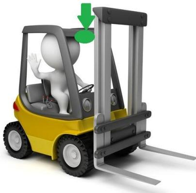
The antenna of anticollision must be installed in the center of forklift. This device measures the distance between its receiver and the operator tag (or another receiver) so it's most important which is mounted in the center of the forklift.
